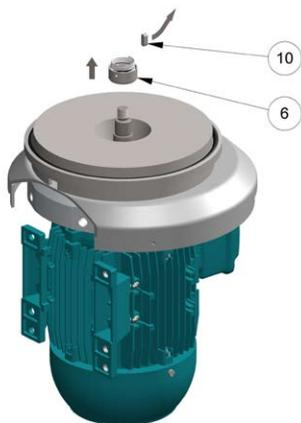
**D** - Remove the key (10) and the rotating part of the mechanical seal (6) inside the cover using two screwdrivers.
