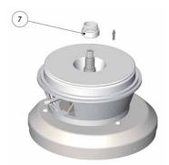
**2<sup>nd</sup> Phase**: extract the rotating part of the mechanical seal (7) by turning the spring anticlockwise.
