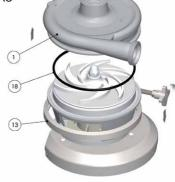
**B** - Loosen the clamp (13) to pull out the pump casing (1) and O-ring (18).
