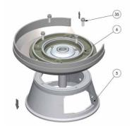
**E** - Turn it over to access the screws (35) which allow you to separate the support (6) from the lantern bracket (5).
