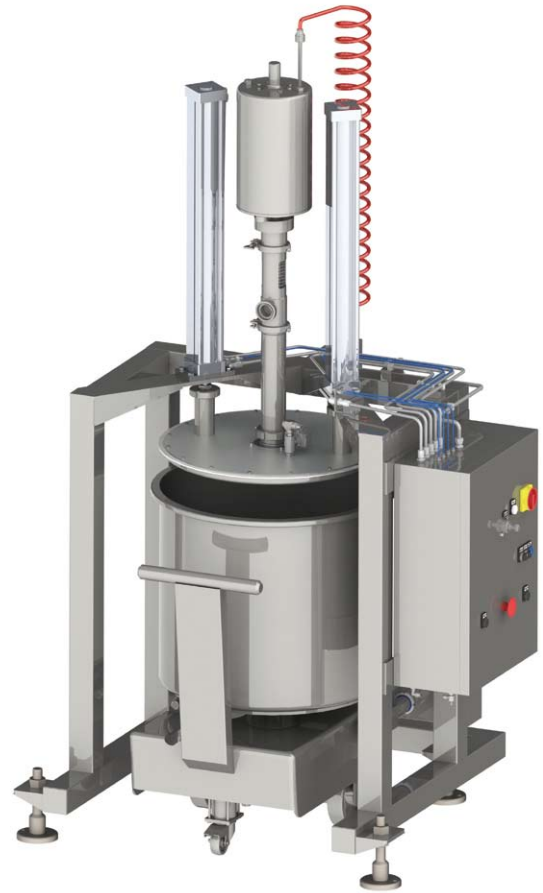
Unit with double pneumatic pistons for vessels with a diameter exceeding 700 mm, including an air operated piston pump and scraper plate. For mixtures, jams, creams etc... to be transferred after processing.
